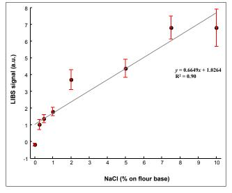
Figure 3. Calibration line showing the relationship between the LIBS Na/K peak integral ratio as a function of NaCl content on dry flour base. The error bars represent the errors from triplicate experiments.
