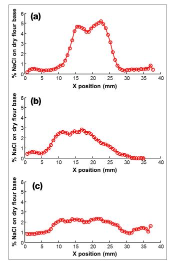
Figure 4. Measured NaCl gradients for bread of zero days, one day and four days old [(a), (b) and (c), respectively].
