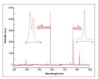
Figure 2. Typical LIBS spectrum of bread. The insets show the relevant spectral regions for sodium and potassium.
