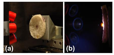
**Figure 1.** (a) Bread sample with salt-rich region, indicated by the purple colour in the centre. (b) Photo taken perpendicular to the bread sample, showing the laser-induced plasma plume.
