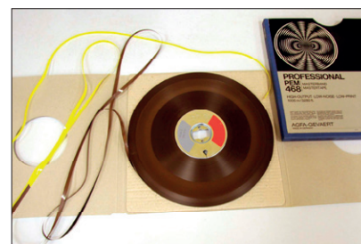
Figure 1. A typical reel tape, with the so-called leader tape (seen here as a red tape attached to the beginning and which carries no information) before the magnetic tape.
