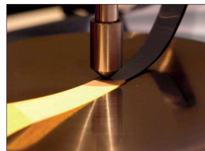
Figure 3. Acquisition of the FT-IR spectrum of a magnetic tape (information side below) in an ATR/FT-IR spectrometer (Spectrum 100, PerkinElmer Ltd). This figure is reproduced from the ICOM-CC publication with permission.
