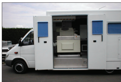
Figure 5. TD-MS/MS instrument mounted in a van.
