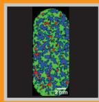
StreamLine<sup>™</sup> Plus image of a pharma-ceutical tablet acquired in less than 4 minutes
